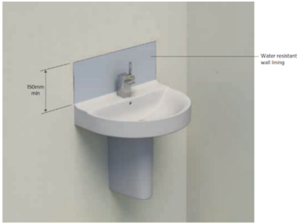
Figure 58: Waterproofing of basin
