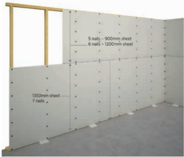
Figure 31: Nail fixing to walls (single nails)
